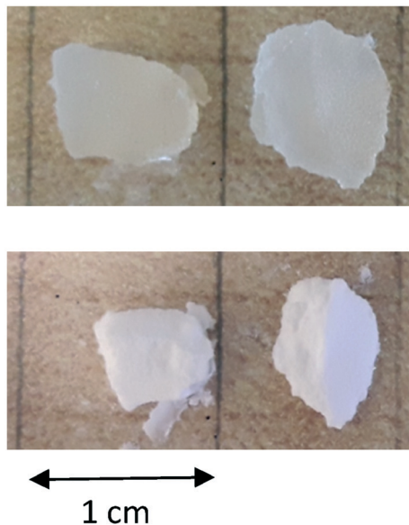
Fig. 7 Images of the PE gels before (top) and after (bottom) the removal of toluene by drying.
